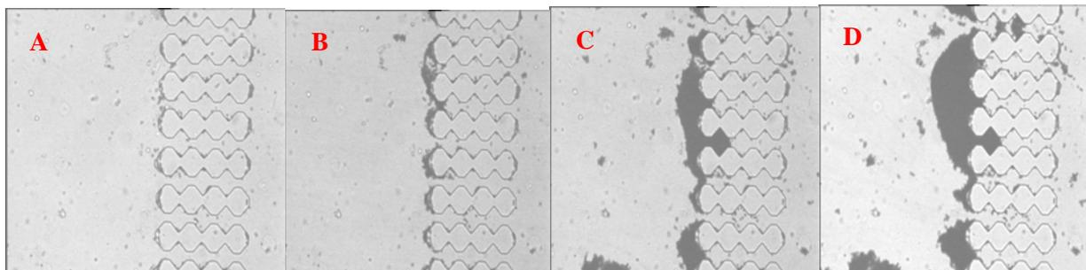
**Figure 4:** Observation of particle capture after a conditioning of the micro-separator with ultrapure water, leading to the progressive obstruction of the microchannels, and then formation of a filtration cake. Image A at  $t_0 + 1$ min, image B at  $t_0 + 20$  min, image C at  $t_0 + 45$  min and image D at  $t_0 + 90$  min.
