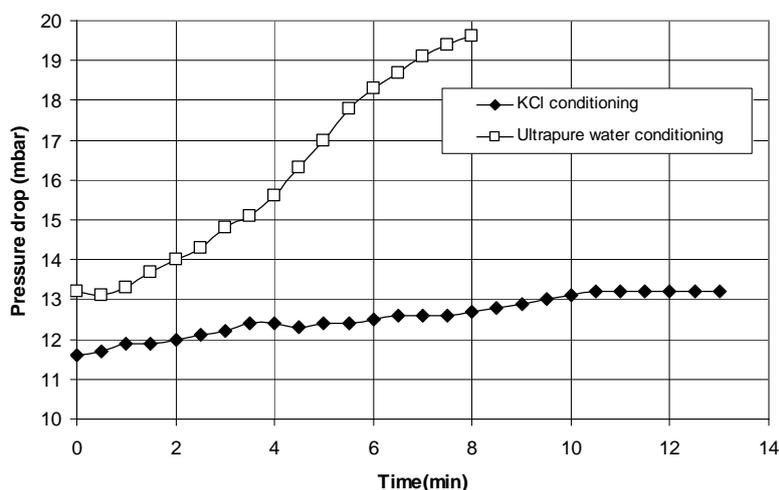
**Figure 6:** Time evolution of the micro-separator pressure drop for two filtration experiments. Diamonds: experiment performed after a PDMS conditioning with a saline solution. Squares: experiment performed after a PDMS conditioning with ultrapure water.
