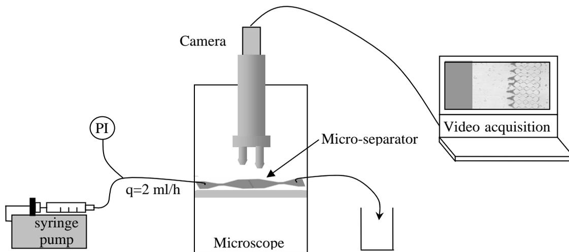
Figure 2: Sketch of the experimental set-up.
