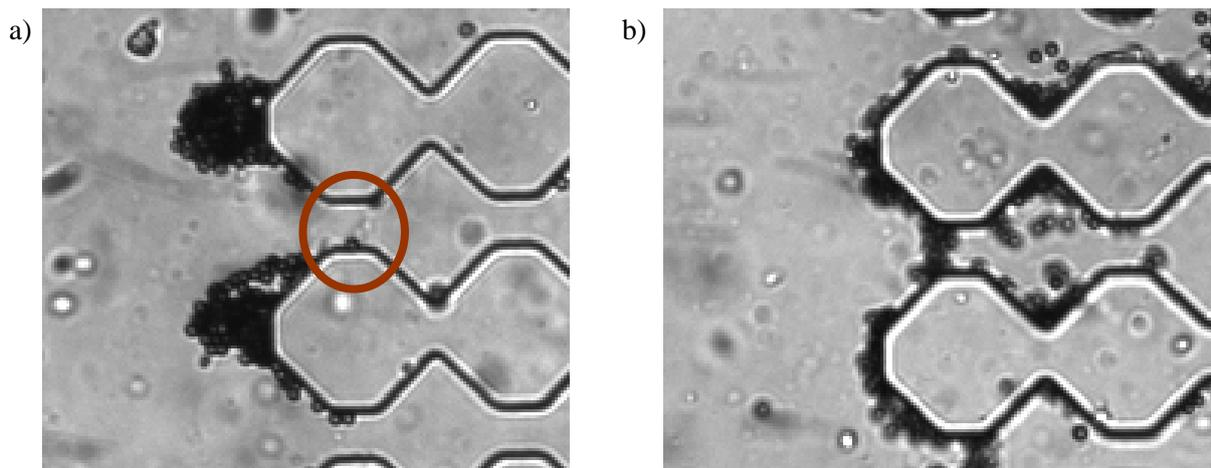
**Figure 5:** Observation of the first stages of the particle capture. a) after a PDMS conditioning with a KCl solution (image taken 1 min after the beginning of the filtration experiment), b) after a PDMS conditioning with ultrapure water (image taken 30 s after the beginning of the filtration experiment). The formation of arches at the entrance of microchannels is clearly seen in image b), whereas such a capture is not seen in a).
