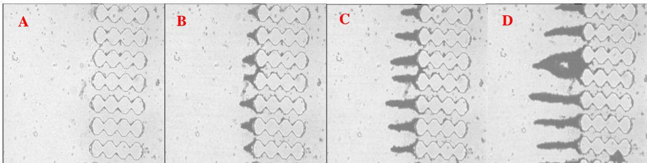
**Figure 3:** Observation of particle capture after a conditioning of the micro-separator with a KCl solution, leading to the formation of dendrites. Image A was taken at  $t_0 + 1$ min (at  $t_0$ , the suspension starts flowing into the microchannels), image B at  $t_0 + 20$  min, image C at  $t_0 + 45$  min and image D at  $t_0 + 90$  min.
