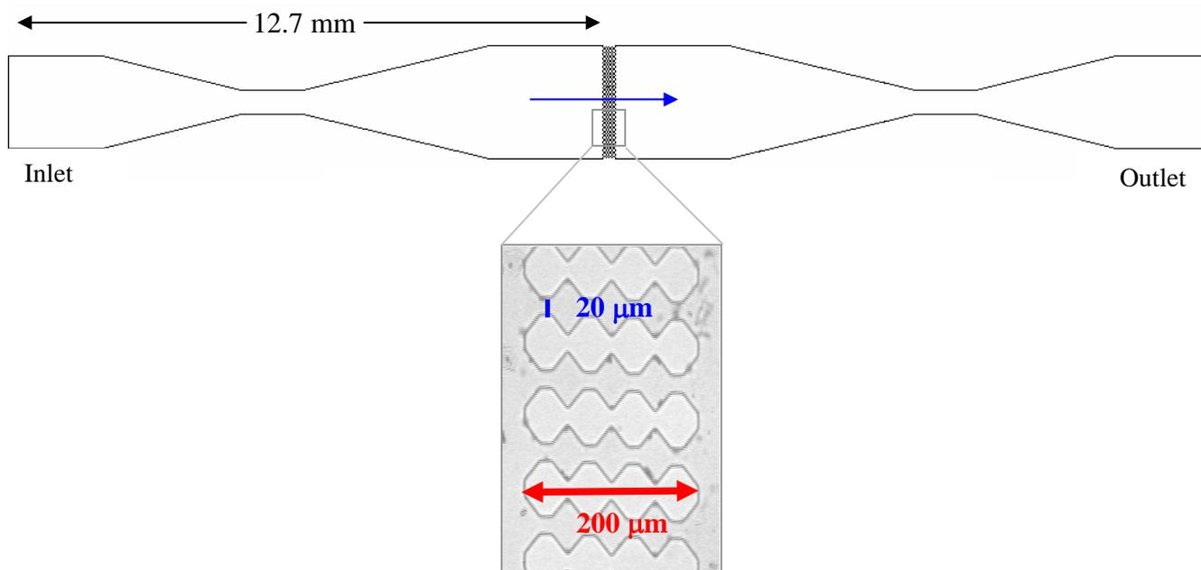
**Figure 1:** Sketch of the PDMS micro-separators (top) with an image centered on some of the microchannels (bottom). The whole filtering part of the device consisted of a parallel arrangement of 27 microchannels.
