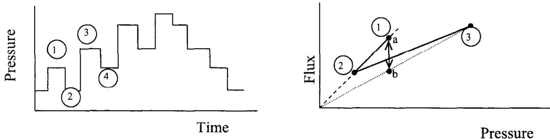
Fig. 2. Pressure vs. time, pressure step used to measure the critical flux, and corresponding flux vs. pressure, the flux of step 4 is included on the segment a-b.
