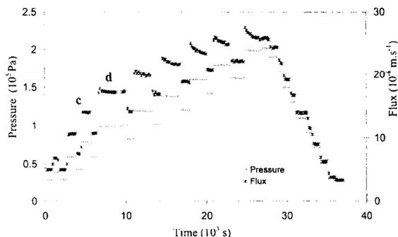
Fig. 3. Flux and pressure vs. time at a crossflow velocity of  $0.98 \text{ m}\cdot\text{s}^{-1}$  with a PVC latex concentration of  $7.1 \times 10^{-4} \text{ g}\cdot\text{L}^{-1}$  without salt. c and d represent the zone where the critical flux appears and are represented in the figures that follow.
