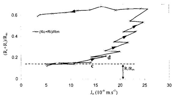
Fig. 5. Evolution of the resistance along the increased and decreased pressure steps; cross corresponds to  $(R_c + R_i)/R_m$  vs. water flux  $J_0$ ; c and d correspond to the zone of the critical flux.
