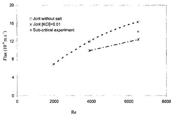
Fig. 6. Critical flux  $J_{\text{crit}}$  vs. the Reynolds number for the filtration of PVC latex with a concentration of  $7.1 \times 10^{-4} \text{ g.L}^{-1}$  with and without KCl; the subcritical flux experiment was run without salt during 8 h without fouling.
