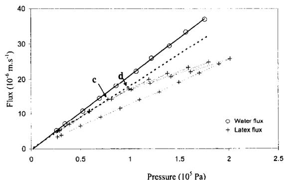
Fig. 4. Relationship between applied flux and transmembrane pressure plotted as flux vs. transmembrane pressure for the filtration of water (circle) and of PVC latex at  $7.1 \times 10^{-4} \text{ g}\cdot\text{L}^{-1}$  (cross) without salt; the crossflow velocity is of  $0.98 \text{ m}\cdot\text{s}^{-1}$  ( $R_e = 6507$ ). The dotted line corresponds to the permeability measured on the first points of the filtration of latex; points c and d corresponds to the range of critical flux.
